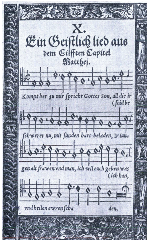
Figure 3 Notes, staves and borders are printed using wood-block (Hyatt King 1968, p.35)
