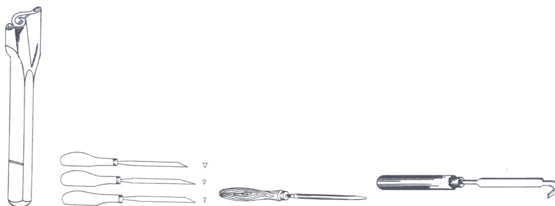
Figure 5 Engraving Tools: a treble clef punch, three tint gravers, a burnisher and a double scorer (Ross 1970, pp.17, 19, 20)
